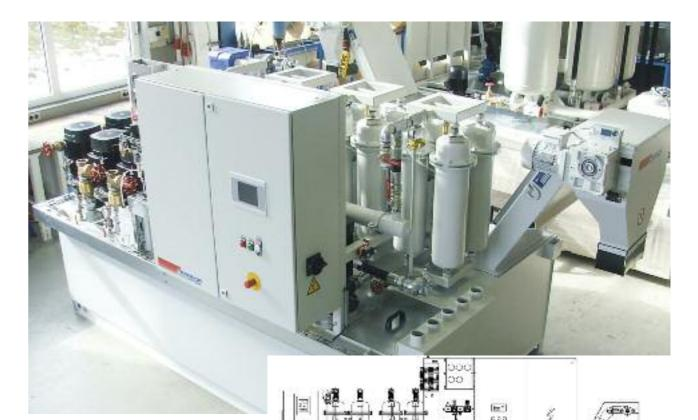
By utilizing so called "island solutions", groups of machines can be connected to one filter unit. These "small centralized systems" are offering concepts which can be adopted to customer specific
