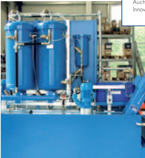
*TRANSOR system including integrated drag conveyor and automatic sludge treating device, with water cooling. Flow rate 100–150 l/min, tank volume 1,500 litres.*
